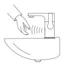
Indicator light fast flush 15 times (in 2 seconds) Then begin auto adjust to your hand distance. Note: Do not move your hand which before the sensor during the adjusting.
