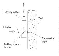
Step seven: When you install the battery case holder, if the wall is not smooth, please use the expansion pipe and self-tapping screw.
