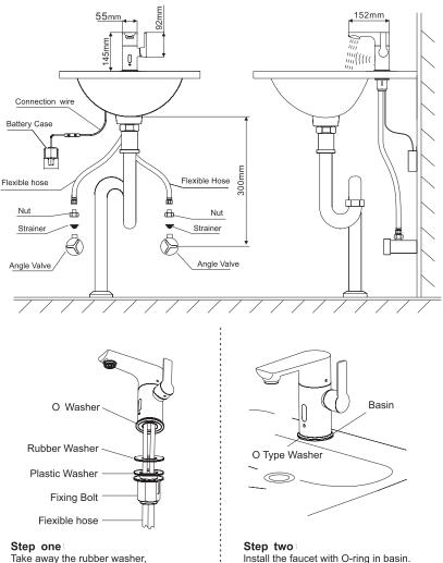
Take away the rubber washer, plastic washer and fixing bolt.
